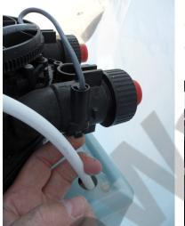
2) Unclip the Turbine Sensor from the rear port. Gently push the clip and it will pull out easily
