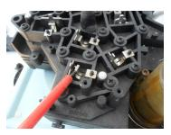
7) With a small screwdriver un-hook each of the stainless steel springs. Note some springs will be doubled. i.e. One on top of the other. Do not attempt to remove the springs off their seating pin
