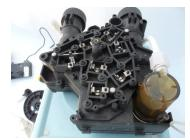
6) Undo the Connection of the Brine tube to the air-check valve and just push to one side leaving full access to the top plate and springs
