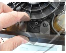
16) Now replace the Control Panel but ensure that the contact switch arm at the back is held in so that it is free of the Main cog and this allows the control panel to clip into place. Be VERY CAREFUL NOT TO BREAK THE CONTACT ARM
