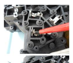
12) Re-engage each of the springs into the hole in the flapper valve. Ensure these are in and secure. You can test by pushing each of the flapper valves towards the spring and ensure the spring closes the valve after tension is released. As in the picture below
