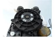
5) Now proceed to remove the motor by removing the two silver covered screws. The Motor and Control Panel can be put to one side leaving clear access to the top plate
