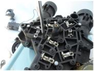
8) Now un-do all of the top plate securing screws. Do not remove the screws as it is best to ensure that the screws go back into the same hole. Not essential but advised so the threads in the plastic moulding beneath are identicle
