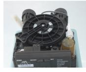
19) Turn on the power. The valve will start to rotate and ERR3 will be in the display. When the valve reaches the home/Service Position the clock will return to time of day.20) Slowly turn on the water supply and check for leaks
